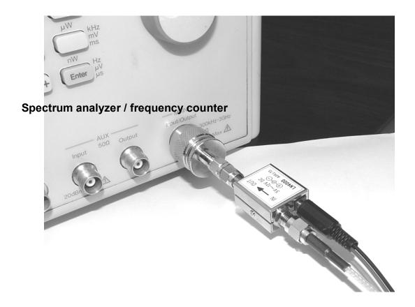
The following example shows sample measurement when LN4000 is used as pot-amplifier for the spectrum analyzer.
