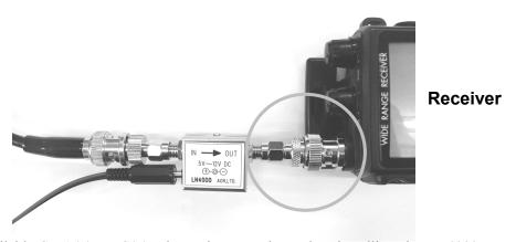
Commercially available SMA(P)-BNC(P) adapter is convenient when installing the LN4000 to a receiver with BNC Jack.
