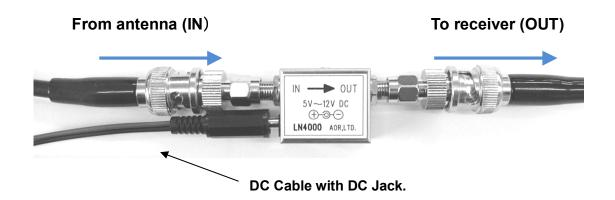
Use supplied DC cable to feed the DC power to the LN4000. Connect wires (black / black-red) to the regulated DC power supply. Black lead should be connected to the negative (-) side of the power supply, and black-red lead should be connected to the positive (+) side of the power supply. Although the LN4000 operates at 12VDC, use medium voltage (8VDC to 9VDC) if power supply is adjustable type. Excessive voltage above 12VDC may damage LN4000.
