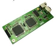
**GPS receiver – GP5001**: Improves the frequency stability of AR6000 from +/- 0.1ppm to +/- 0.01ppm, by using the GPS pulse signal for an accurate time base of the local oscillator circuit.
