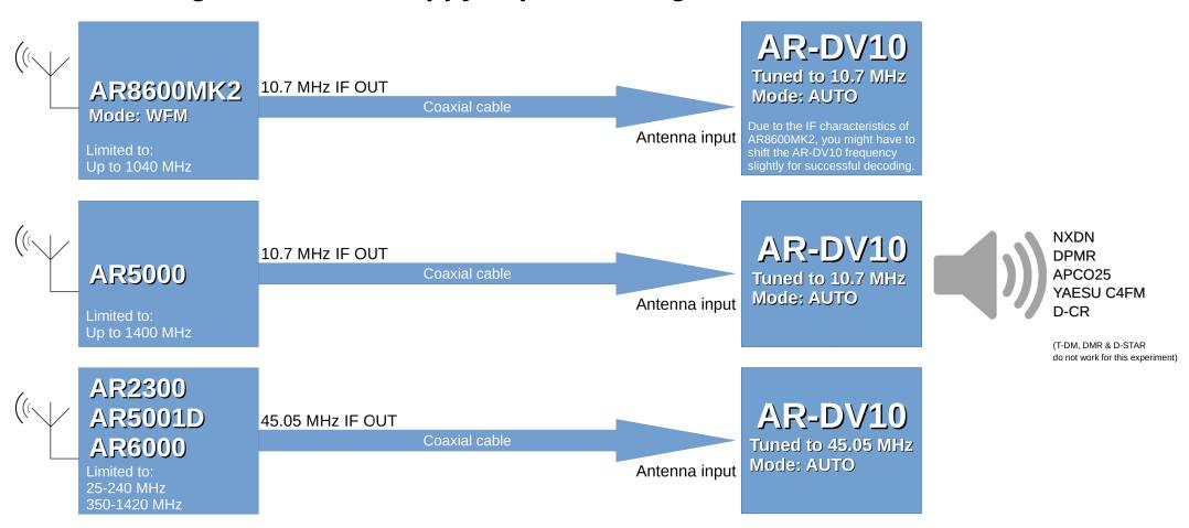
Caution: Do not connect an IF signal which contains voltage, as it might damage the AR-DV10. Some non-AOR receivers such as from ICOM have an IF which carries 9VDC or more. It is your responsibility to check the receiver's manual. AOR can't be held responsible for any damage.
