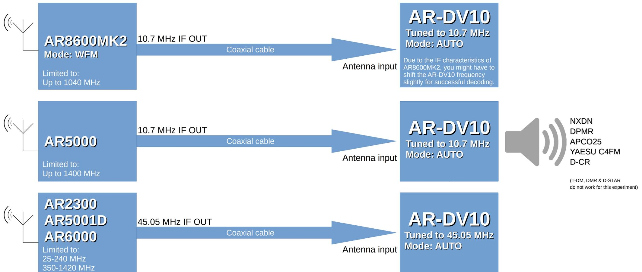
**Caution:** Do not connect an IF signal which contains voltage, as it might damage the AR-DV10. Some non-AOR receivers such as from ICOM have an IF which carries 9VDC or more. It is your responsibility to check the receiver's manual. AOR can't be held responsible for any damage.
