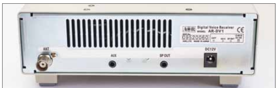
Fig. 1: The AR-DV1's rear panel.
