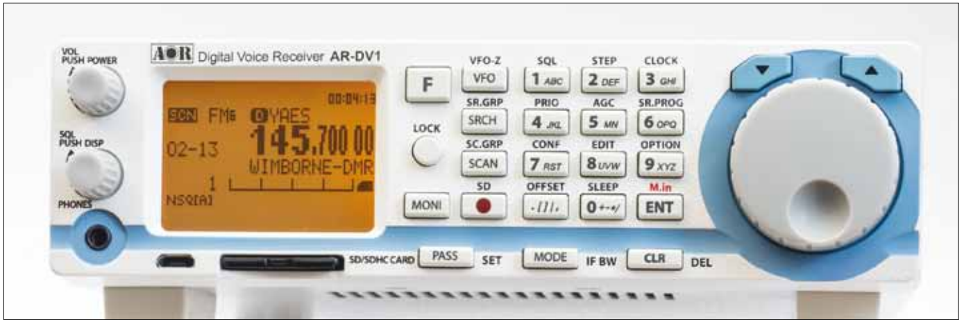
Fig. 2: The AR-DV1's front panel.
