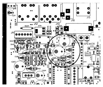
The modification involves the repositioning of C119 and R110 in the audio amplifier output feed as shown in the diagrams above.
