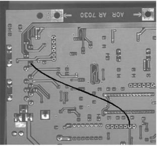
The PCB layout shows the positions of J8 and the remote DIN socket connections. Connect as short a wire as possible between the two points as shown. A ground connection is available on pin 5 of the remote DIN socket (see operating manual).
