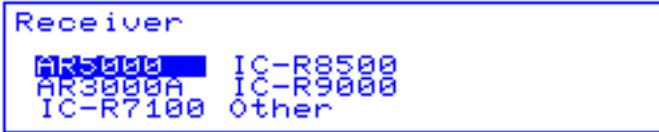
Use the spin wheel dial to highlight "AR5000" then press **ENT**. The legend "AR5000 Connected" will briefly be displayed then the CF readout will display the current receive frequency of the AR5000 and the RX readout will confirm AR5000.
