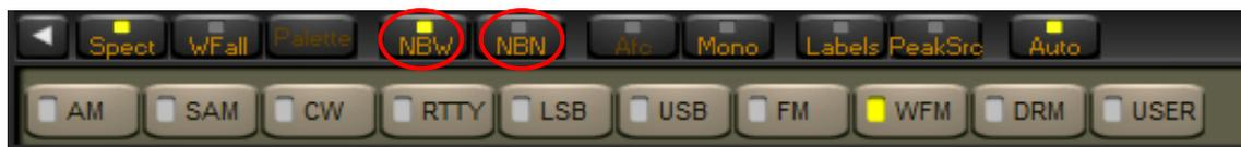
The Narrow NB, operates on the bandwidth selected with the BW buttons (56 kHz, 28 kHz, 14 kHz, etc).
