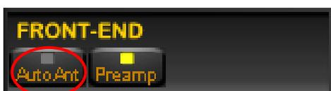
Automatic antenna selection is possible by clicking the "AutoAnt" button in the FRONT-END section of the screen.
