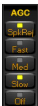
The Automatic Gain Control keeps the audio output at a constant output level, disregarding the input signal power. Three time decay constants can be selected with the buttons "Fast", "Med", and "Low" in the AGC control bar.
