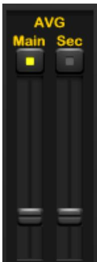
**AVG Main:** Stabilizes the spectrum waveform in the main spectrum / waterfall display. Will also stabilize the waterfall mode. The main spectrum average function and its slider control are active only when the enable button above the slider is enabled.
