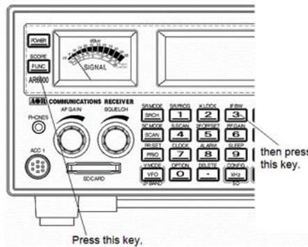
Select a new bandwidth from the list by rotating the sub dial. To accept the new bandwidth selection, press the [MHz] key.
