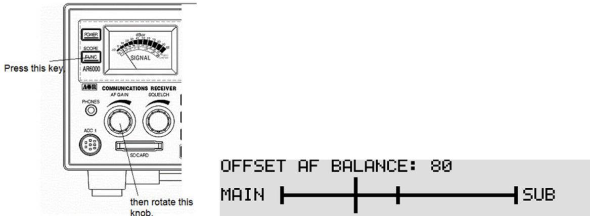
Rotate the AF gain (volume) to the desired audio level for both frequencies.
