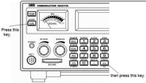
4. When the configuration menu is displayed, press the [DOWN] key seven times to select “SD INFO” in reverse contrast.
