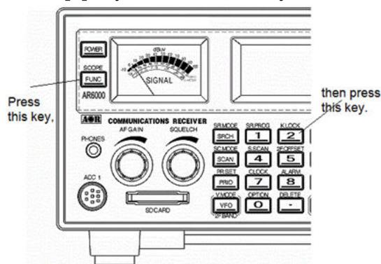
While activated, all front panel keys except the **[FUNC]** key, and **[POWER]** key are disabled to prevent accidental misoperation of the receiver. However, the volume and squelch controls remain operative.
