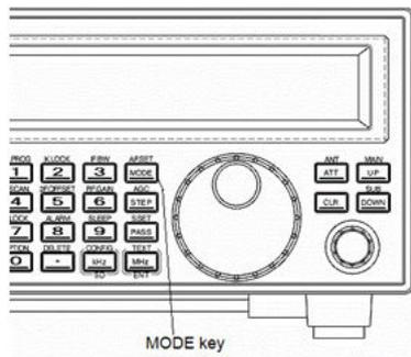
To activate auto mode or reconfirm its selection while in VFO mode, press and hold the [MODE] key for two seconds. “AUTO” will appear above the frequency portion of the LCD.
