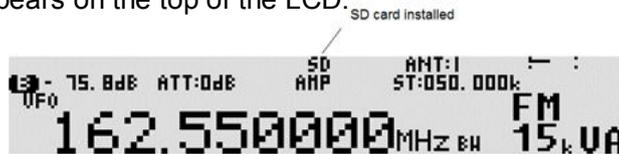
3. Press and hold the [kHz] key for two seconds. Recording will start and the "SD" icon will change to "REC".
