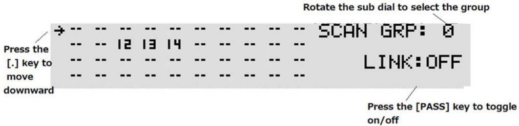
3. To select the memory bank to be linked, enter the memory bank number using the numeric keypad. If the memory bank is between 10 ~ 19, press the [.] key to move the cursor to the second row and enter only the first digit of the memory bank number from the numeric keypad. (Example: If the memory bank is 12, enter "2".)
