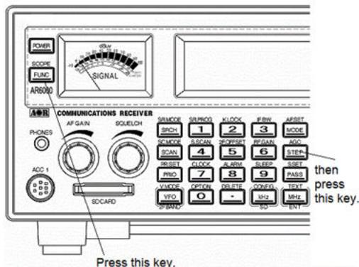
Select a new AGC parameter from the list of “FAST”, “MIDDLE”, “SLOW”, or “OFF (MANUAL)” by rotating the sub dial.
