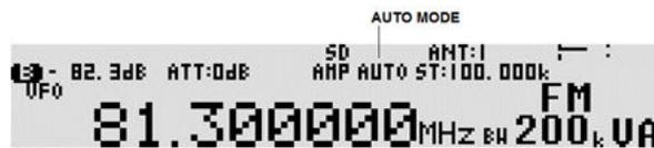
Note: Auto-mode is cancelled as soon as the receive mode, tuning step or other related data are changed. Remember that auto-STEP and auto-MODE are linked, reselect **AUTO MODE** if either have been adjusted and you require the auto band plan selection.
