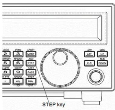
If you wish to change the default tuning frequency step, press the **[STEP]** key. The LCD will display the current frequency step and the blinking “STEP” while waiting for the new parameter. Use the sub dial to select the desired step.
