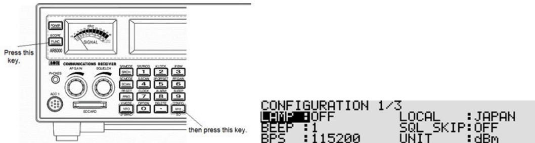
4. When the configuration menu is displayed, press the [UP] key four times to select “SD FORMAT” in reverse contrast.
