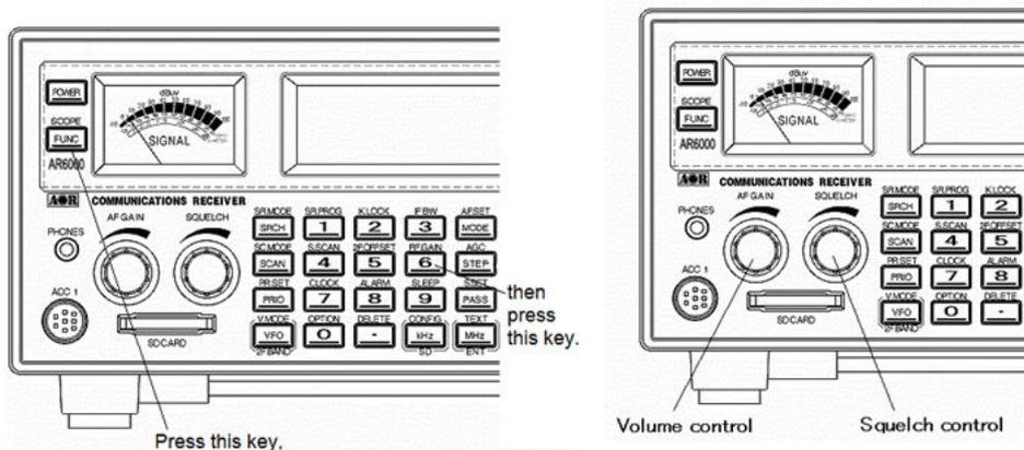
To change the RF gain manually, rotate the squelch knob. To cancel the manual RF gain control, repeat above steps.
