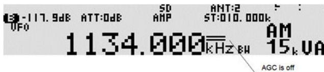
When AGC is set to OFF, the RF gain control can be adjusted.
