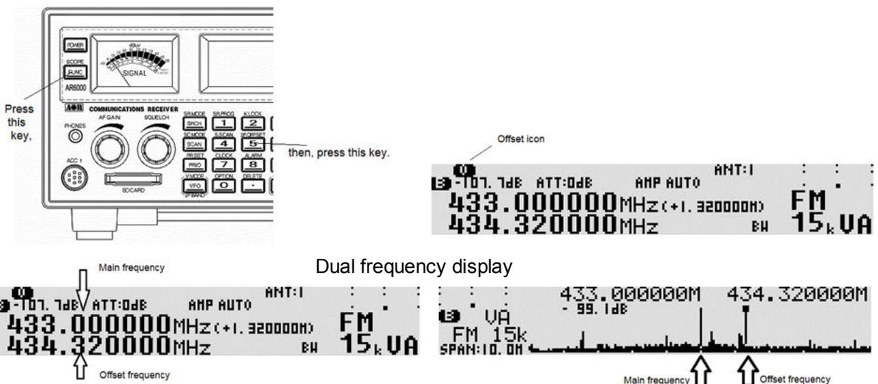
The offset frequencies can also be displayed in the spectrum display mode by pressing and holding the [FUNC] key for two seconds.
