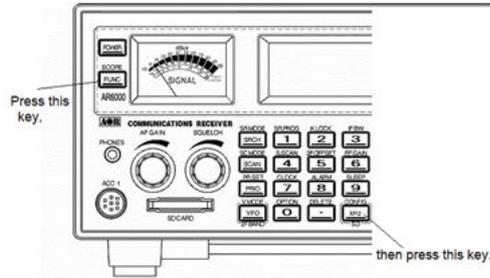
4. When the configuration menu is displayed, press the [UP] key seven times to select "SD INFO" in reverse contrast.
