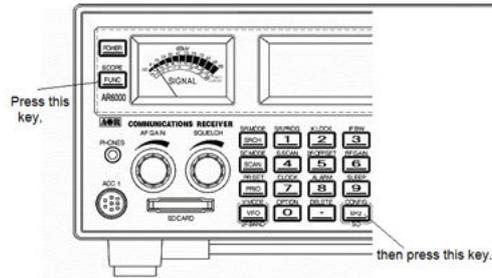
When the “LAMP” is displayed in reverse contrast, rotate the sub dial to toggle the lamp on or off.
