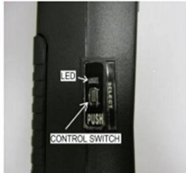
2. Double clicking the **[CONTROL]** switch will toggle through the APCO25 mode (one beep), Voice Inverter mode (two beeps, not available for US consumer model), and CTCSS mode (three beeps).
