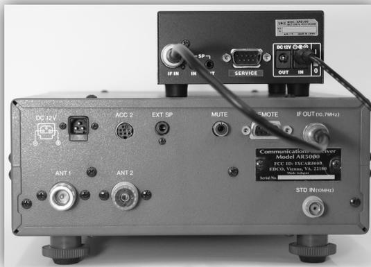
Each unit needs its own power source; therefore you will need to supply the power source for ARD300. If you happen to own the AR8600MK2 receiver, you can use its AC adapter AA8600. (The AA2300 adapter of AR2300/5001D/6000 can be used as well)
