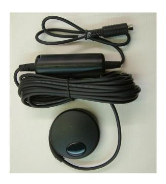
The GP5001 GPS receiver system differs from typical "map based" positional systems. It feeds a highly accurate one-pulse-per-second (PPS) signal to the AR2300/5001D/6000/5700D receiver. The rising edge of the signal is aligned to the start of each GPS second within 1µsec.
