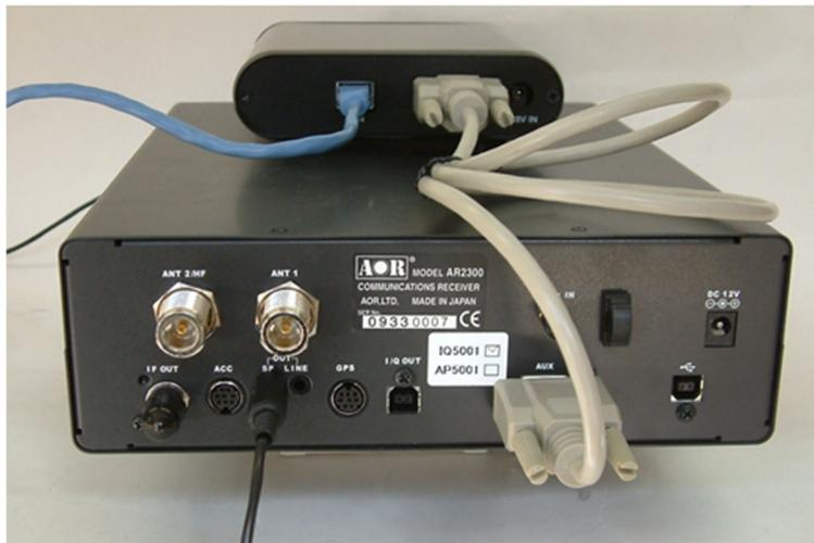
Remarks: On the receiver side, the audio cable can alternatively be connected to the back-panel's LINE output or the front panel's PHONES output. Audio level adjustment is not possible when connected to LINE
